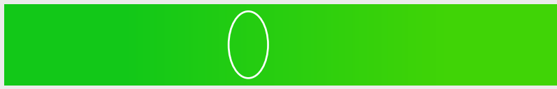
Figure 28. MacAdam Ellipse. Most people cannot discern differences in the greens inside a MacAdam ellipse.
